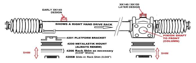
IMPORTANT: NEW RACKS ARE LINE BORED, WHICH ENSURES THE RACKBAR RUNS PERFECTLY BETWEEN THE OIL-LITE BUSHES. THIS IS AN INTERNAL MACHINING PROCESS AND AS WITH MOST XK COMPONENTS MEANS THE RACK CASING MUST BE SHIMMED ONTO THE CHASSIS.
