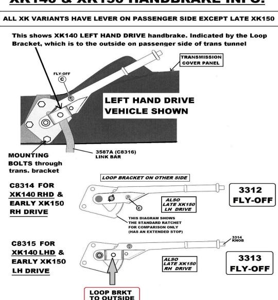
NOTE: THE LOOP BRACKET FACES OUTWARD TO SECURE DROP LINK BAR 3587A TO THE FIRST KNUCKLE JOINT BELOW FLOOR.
